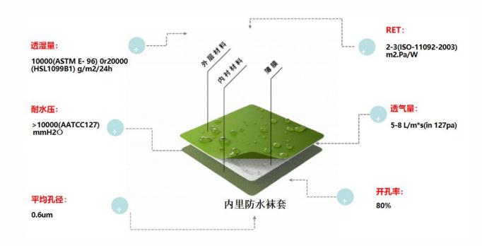
Optimized water resistance with three layers of insurance to provide excellent water resistance.
